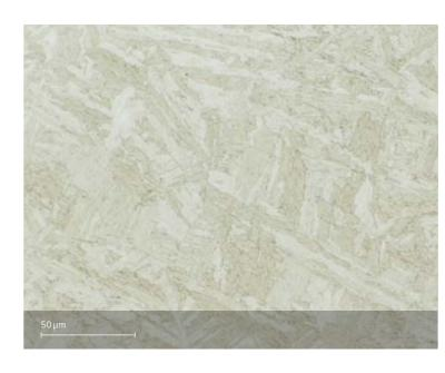
Heat treated microstructure. Etched according to ASTM E407-07, recipe 94.
