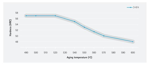
If lower hardness and improved toughness is required, aging temperature can be increased according to figure above.
